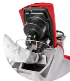
Automatic swing-in of the brush head and automatic squeegee uncoupling when accidentally impacted
